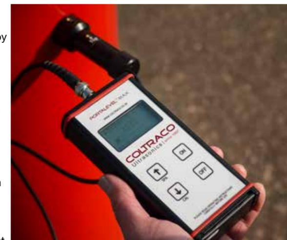
weighing) with accuracy of up to 1.5mm off the true liquid level. The system builds on Coltraco Ultrasonics 30 years' experience in designing, manufacturing and supporting ultrasonic liquid level indicating equipment, in 108 Countries and numerous market sectors and environments. The development programme was born out of the desire to further improve on Coltraco's existing eight designs and taking on board feedback and opinions of our customers.
