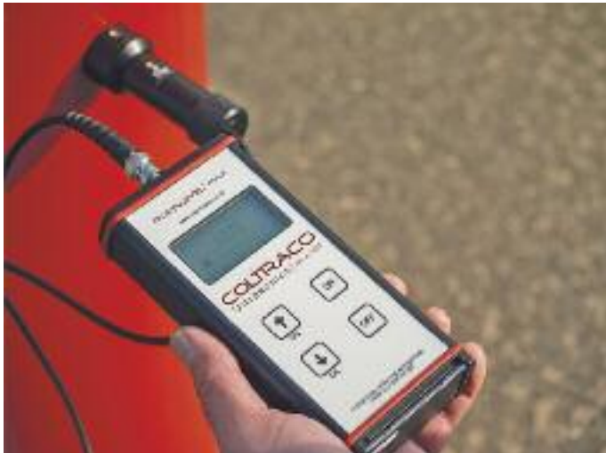
The Coltraco Portalevel® MAX is a leading handheld ultrasonic liquid level indicator for testing most common extinguishing agents
